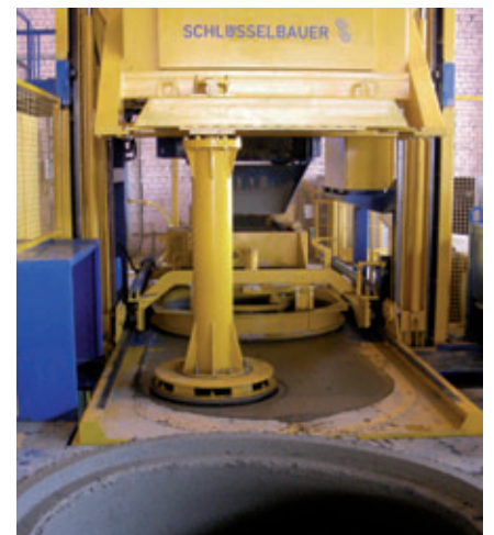
Production cycle: Pallet is fed in, mould filled and after compacting the cone is released from the mould and transported out of the machine.
