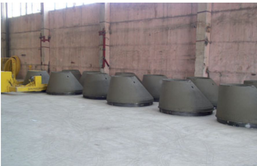
Cones in the curing area of the production building at OOO <<SMK-50>>
