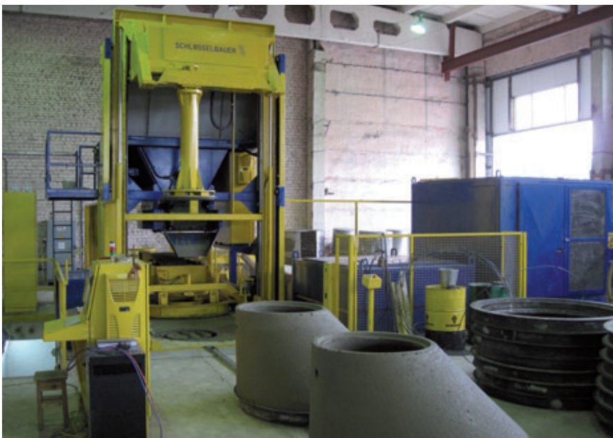
Production of manhole cones at OOO <<SMK-50>> using the new production plant Magic from the company Schlüsselbauer.
