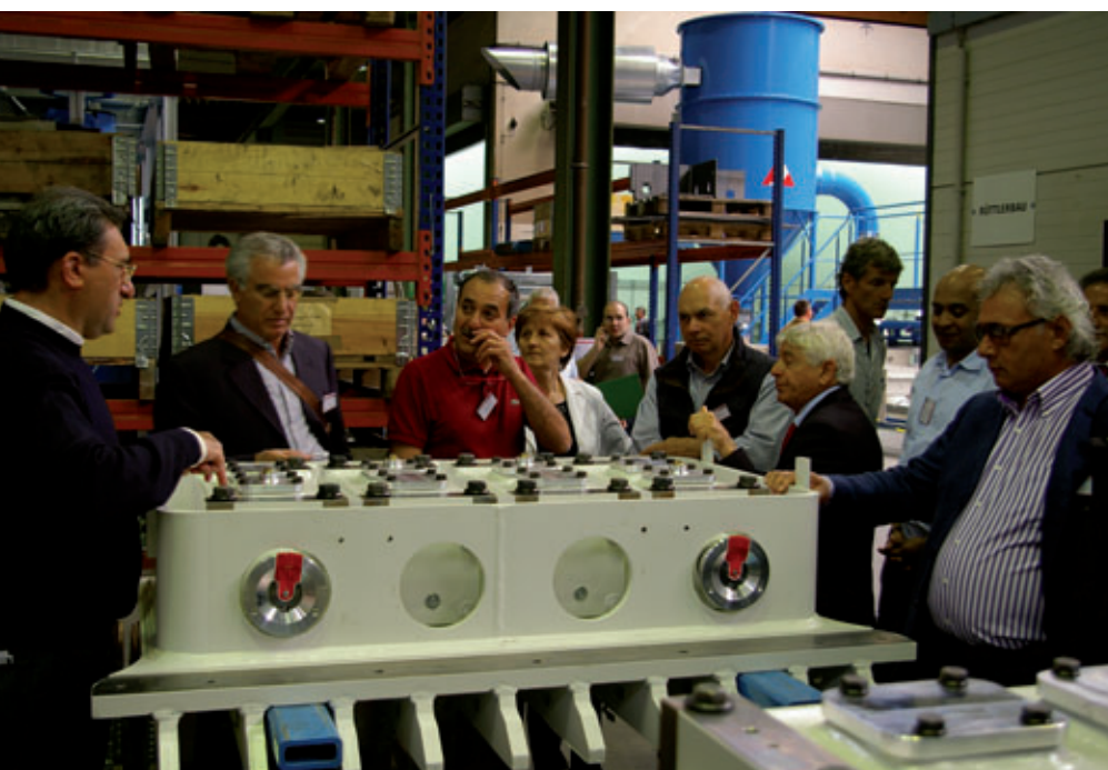
The visitors were particularly interested in the new oil-bath vibrator, which works almost completely maintenance-free. The visitors were particularly interested in the new oil-bath vibrator.
