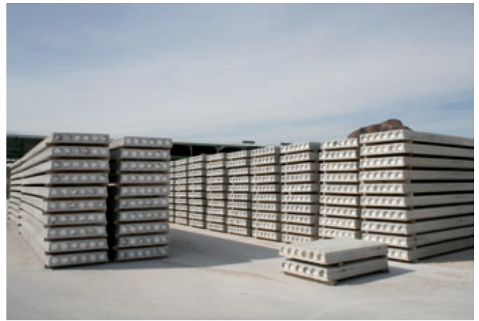
The prestressed hollow-core slabs manufactured on plants by Elematic and Prensoland are produced on a total of 14 lines, each of which is 165 m in length
