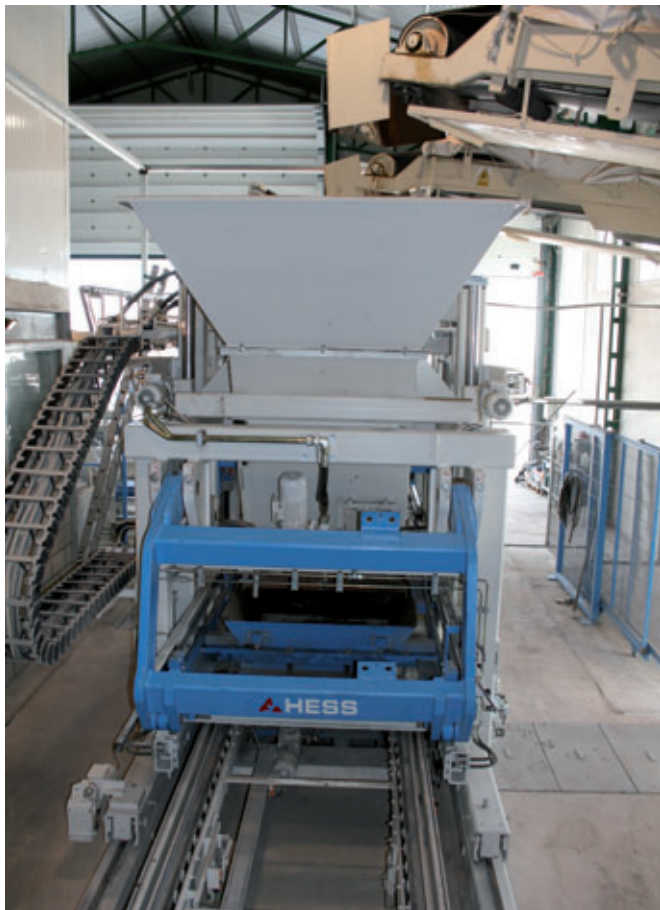
The RH1500-2 VA concrete block making machine is fed by a conveyor belt
