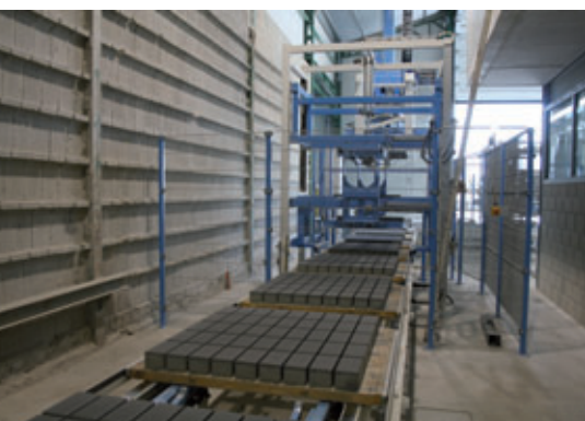
The cured products on the way to the stone releaser and squeezer
