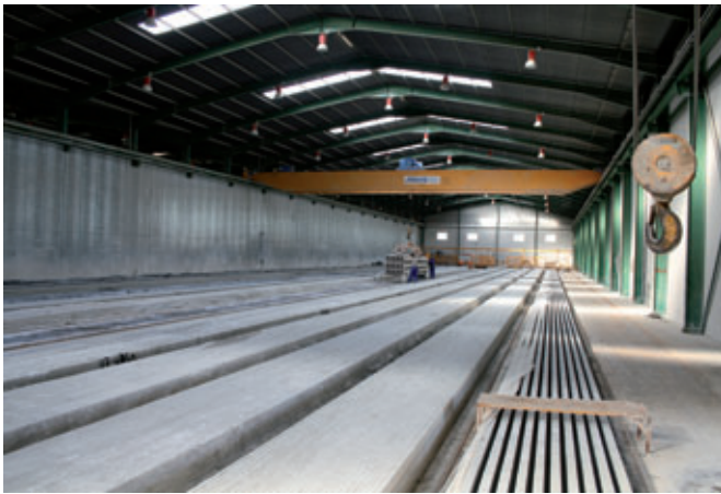
The prestressed hollow-core slabs manufactured on plants by Elematic and Prensoland are produced on a total of 14 lines, each of which is 165 m in length
