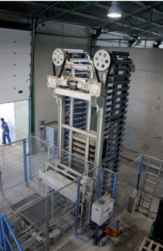
Following manufacture the product is transferred to the V-belt conveyor via a lowering device and transported to the elevator
