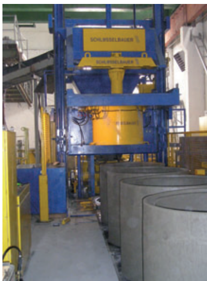
Wet products in the „parking area“ and before the transport to the curing area
