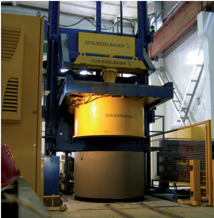
The company Kauno Gelzbetonis has invested in the new Schlüsselbauer production plant for the production of manhole rings and cones
