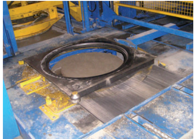
Production procedure: pallet is fed in, concrete is poured into the mould, after setting the manhole cone is removed from the pallet and pushed out of the machine
