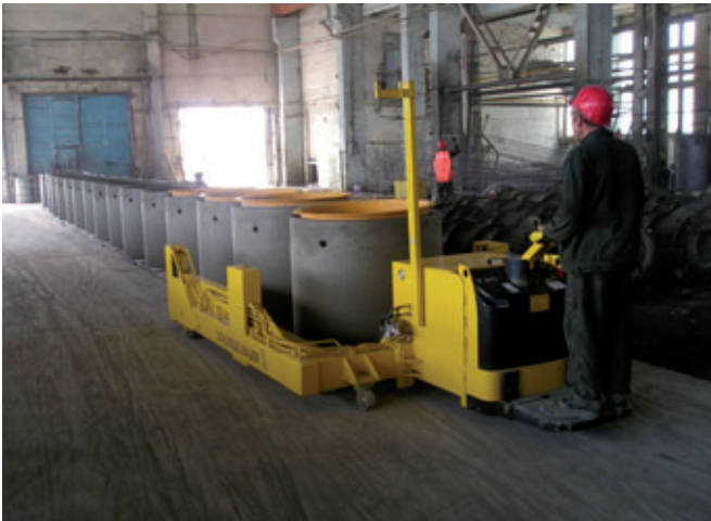
The Magic 1501 at the company Kauno Gelzbetonis is laid out to be operated by two machine operators
