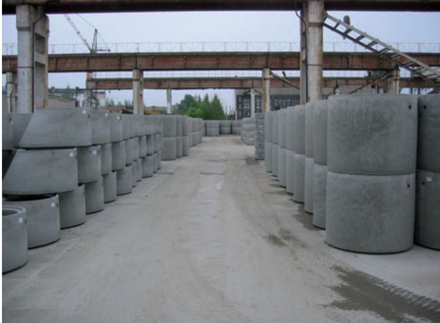
Modern manhole components for civil engineering in Lithuania – in the picture cones and manhole rings at the company Kauno Gelzbetonis
