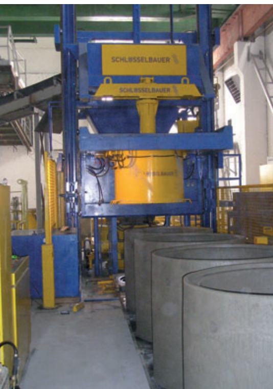
Wet products in the „parking area“ and before the transport to the curing area
