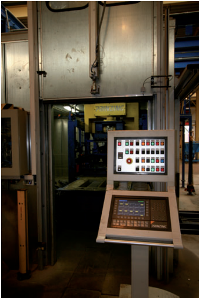
All the production parameters can be viewed on the control desk monitors
