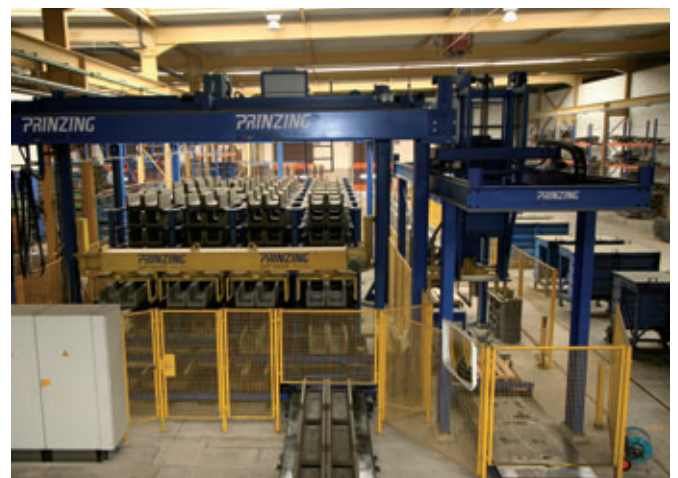
The ingenious design of the crane robot and rack system means that only a small amount of room is required for the entire plant
