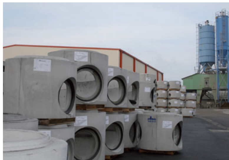
The storage area for manhole components at Stradal
