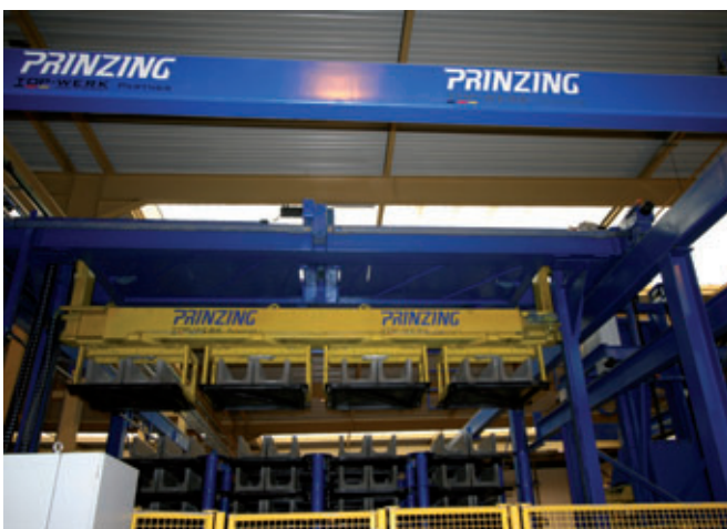
The ingenious design of the crane robot and rack system means that only a small amount of room is required for the entire plant
