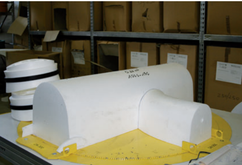
The construction of a negative mould piece – In the photo an inlet DN 200 in a main channel DN 300.
