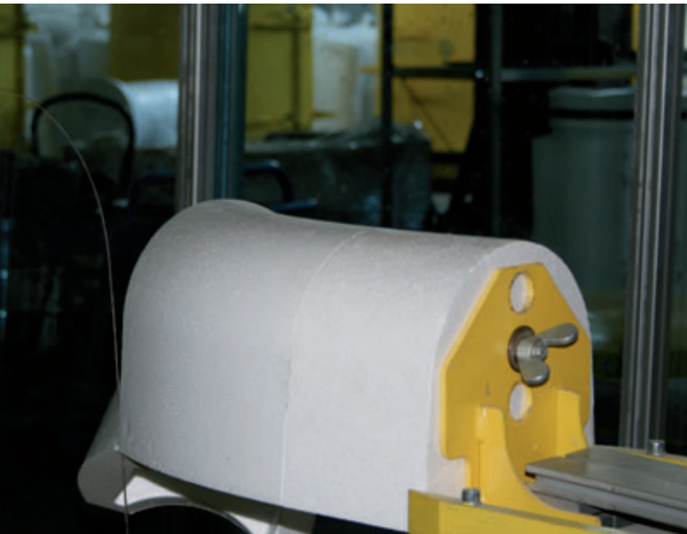
The „three dimensional cut“ of an EPS mould.
