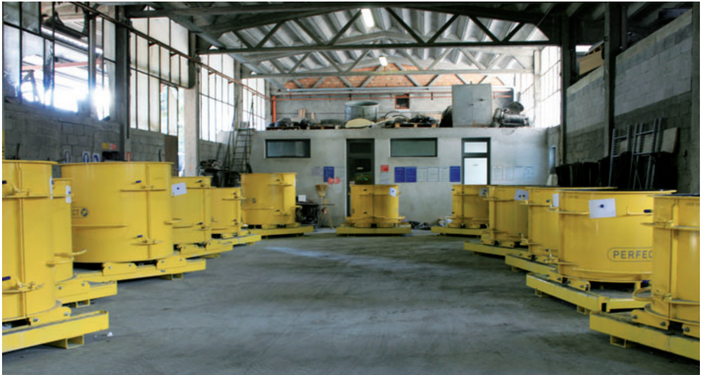
View of the production building at Buzzella Ennio SRL: Perfect moulds for the production of manhole bases DN 1000 and DN 1200.
