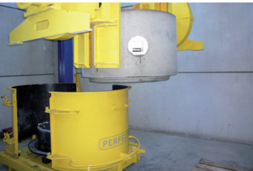
De-moulding of the cured monolithic manhole base.
