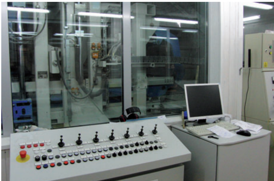
Fig. 2: The heart of the plant is a Hess RH 1500-2 VA with a board size of 1400 x 950 mm
