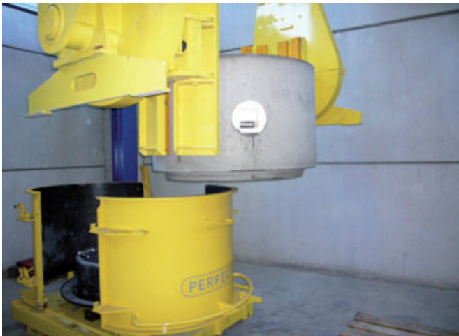
De-moulding of the cured monolithic manhole base.
