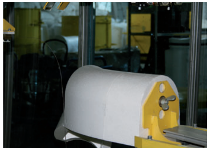
The „three dimensional cut“ of an EPS mould.
