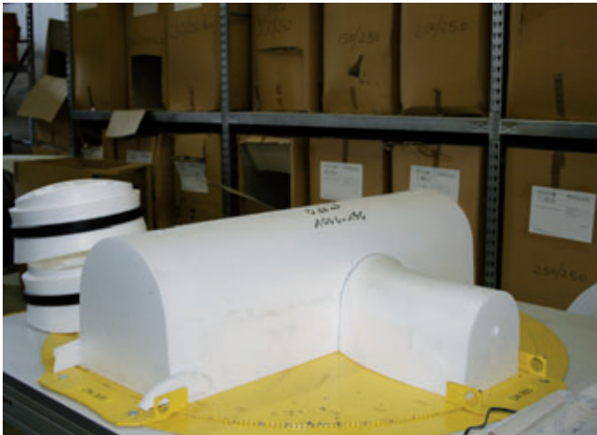
The construction of a negative mould piece – In the photo an inlet DN 200 in a main channel DN 300.
