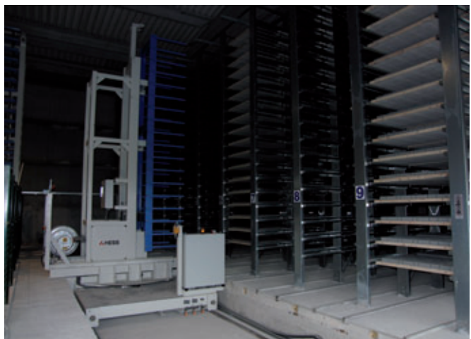
Fig. 3: The finger car takes the production boards to the Rotho curing rack installed opposite the plant
