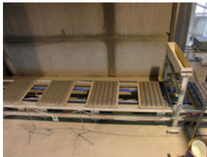
Fig. 4b/c: After separation, the products are transported to the packet assembler by an accumulation pawl conveyor
