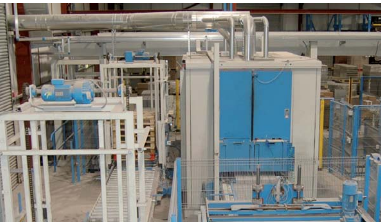
Layer conveyor for the shot-blasting machine
