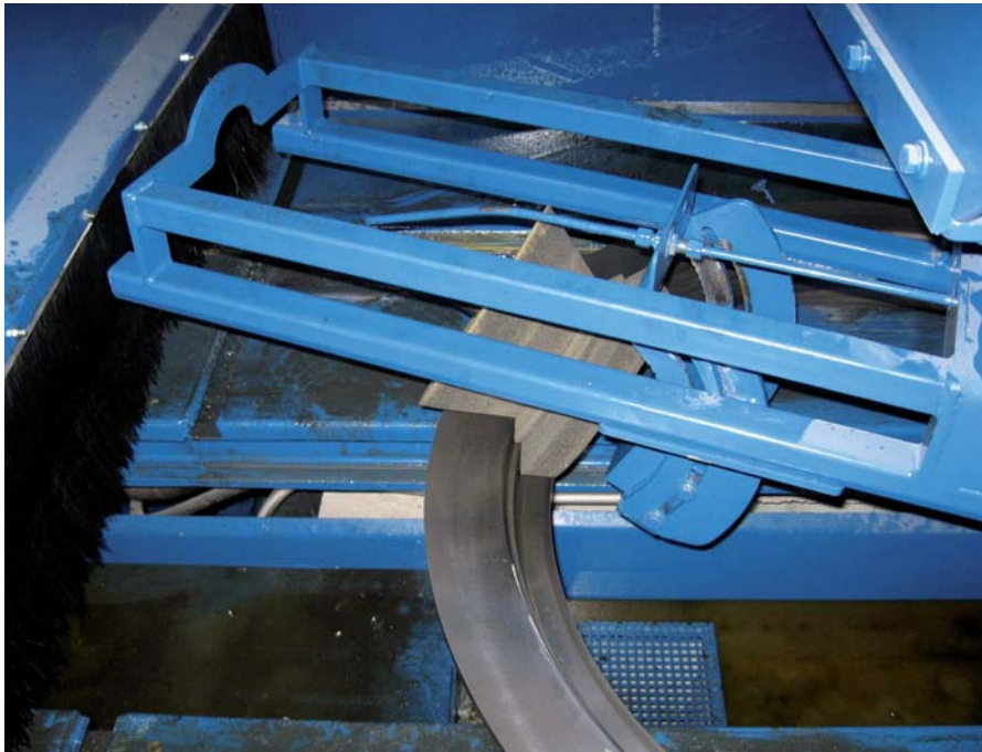
Oiling by use of a sponge: No drizzle, no contamination of the working area.
