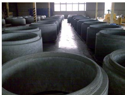
Manhole cones and manhole rings within the curing area of the company.
