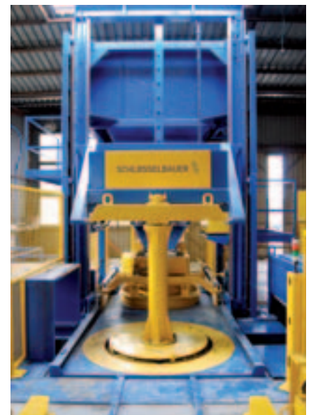
The Schlüsselbauer Magic 1501, designed for one-man operation, during production.
