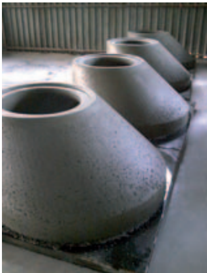
Manhole rings with dimensions of 1000 and 1200mm and total heights of 500, 750 and 1000mm are produced.
