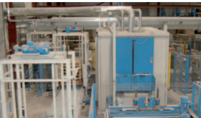
Layer conveyor for the shot-blasting machine
