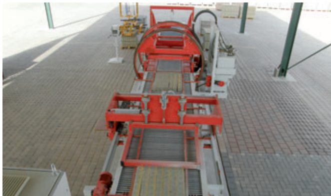
An accumulating roller chain conveyor and layer pusher then insert the products into the calibrating machine
