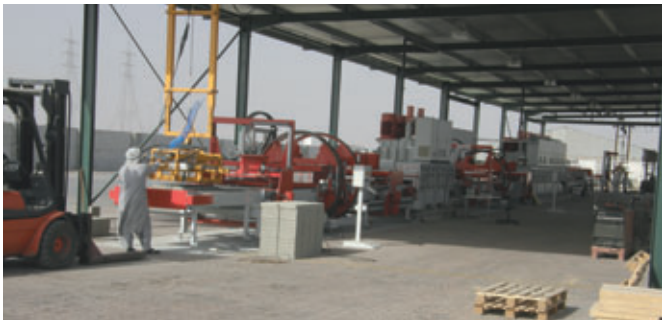
At the outset of the finishing plant, there is a belt conveyor permitting the block layers to be positioned semi-automatically with the customer's own clamp
