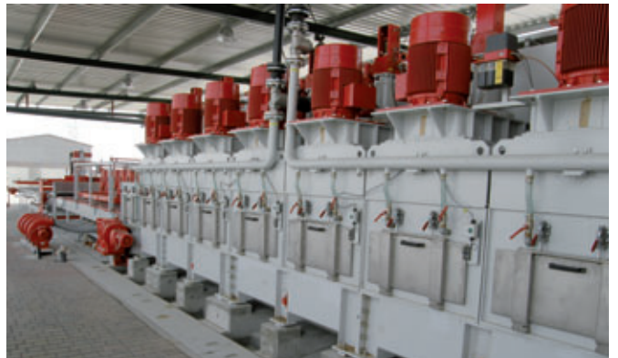
The grinding machine possesses 8 stages for milling, polishing and grinding
