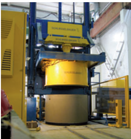
Production of manhole rings with different dimensions at the concrete works Kauno Gelzbetonis and Vilniaus Gelzbetoninis Konstrukcijs Gamykla Nr. 3.
