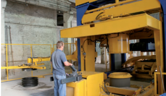
Transport of a manhole out of the Magic production plant at the concrete works Marijampolés Gelzbetonis.
