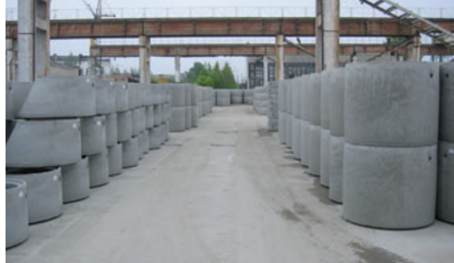
Modern manhole components for use in civil engineering in Lithuania -This photo shows manhole cones and manhole rings at the company Kauno Gelzbetonis.
