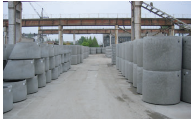
Modern manhole components for use in civil engineering in Lithuania -This photo shows manhole cones and manhole rings at the company Kauno Gelzbetonis.
