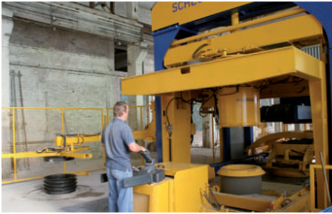
Transport of a manhole out of the Magic production plant at the concrete works Marijampolės Gelzbetonis.
