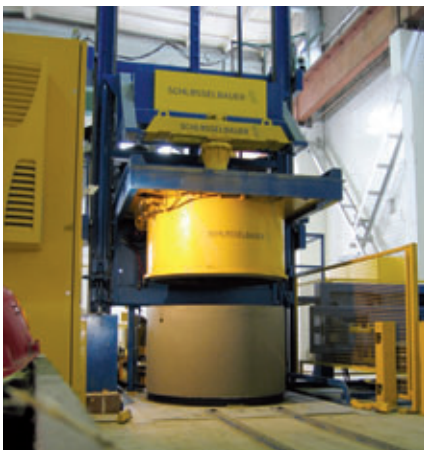
Production of manhole rings with different dimensions at the concrete works Kauno Gelzbetonis and Vilniaus Gelzbetoninis Konstrukcijos Gamykla Nr. 3.
