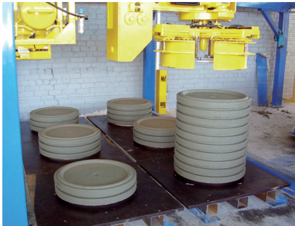
Production and handling of covers by use of the Ringmaster automatic stacking system.
