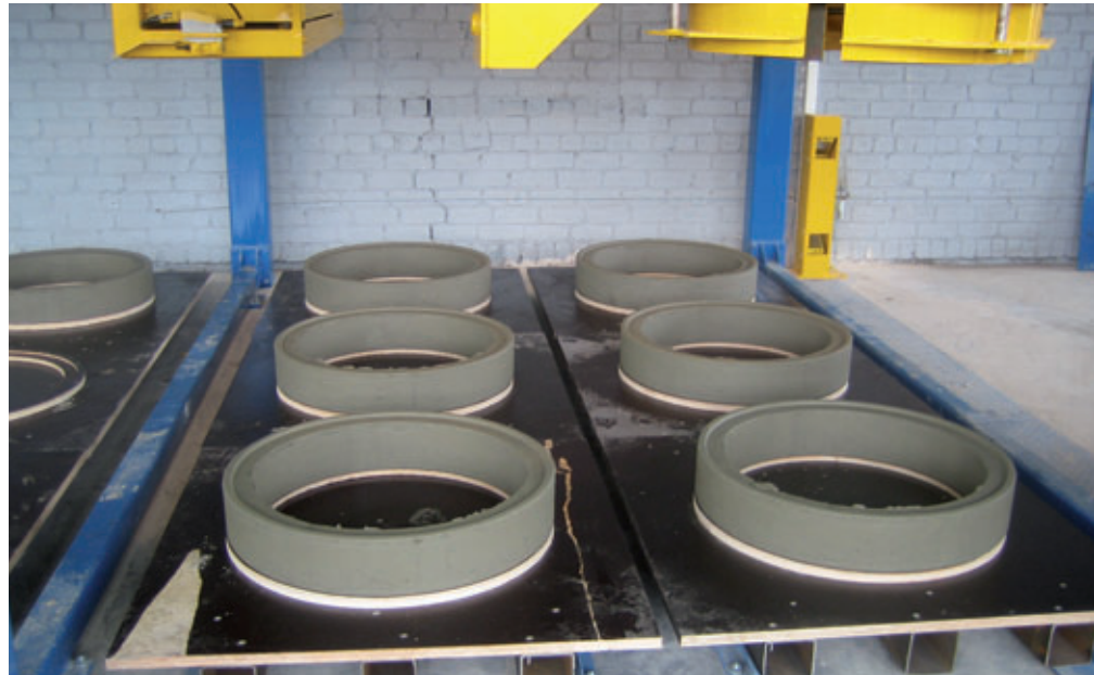
Adjustment ring with rebated joint DN 700 from the Ringmaster production at the company JSC Gelgaudiskio Gelzbetonis
