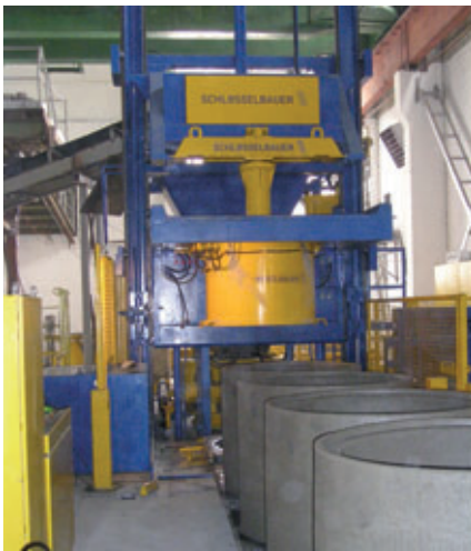
Adjustment ring with rebated joint DN 700 from the Ringmaster production at the company JSC Gelgaudiskio Gelzbetonis
