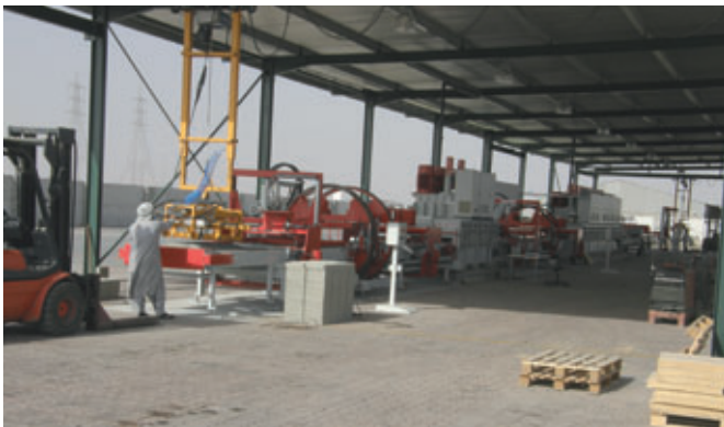
At the outset of the finishing plant, there is a belt conveyor permitting the block layers to be positioned semi-automatically with the customer's own clamp
