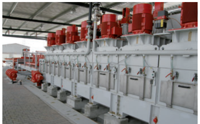
The grinding machine possesses 8 stages for milling, polishing and grinding
