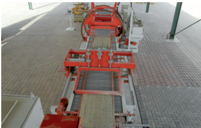
An accumulating roller chain conveyor and layer pusher then insert the products into the calibrating machine
