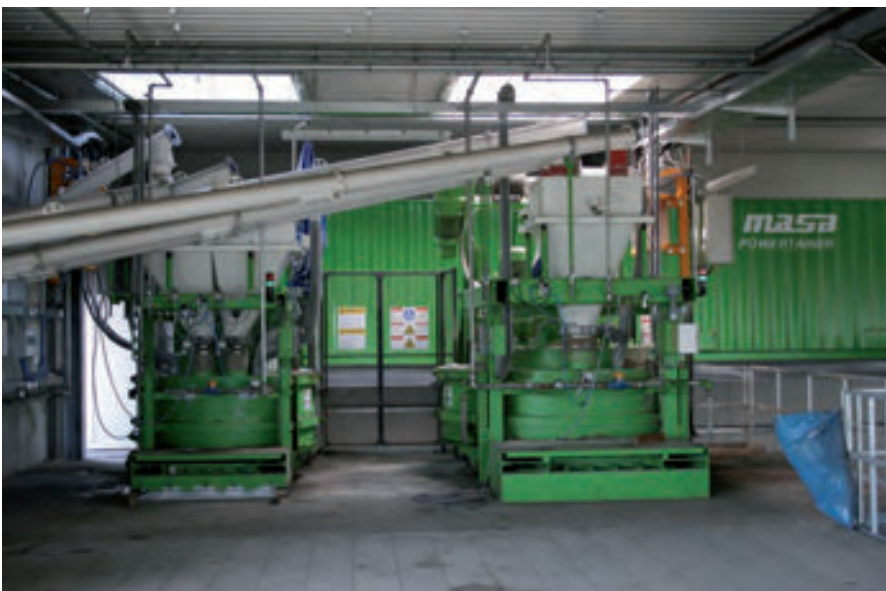
Two horizontal compulsory mixers by Masa produce facing and core concrete for the block production (shown in the picture with a Masa Powertainer).
