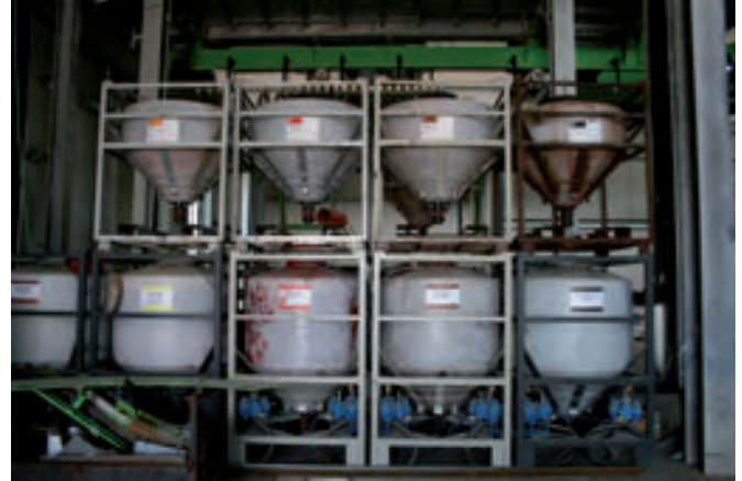
Individual colouring takes place via a 4-colour dosing unit.
