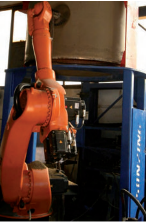
Fig. 5: Milling the connections on the milling centre
