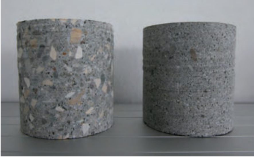
Fig. 3: Drilling cores \varnothing 90 mm, length 100 mm from the manhole bottoms, left normal concrete, right PRIMUS manhole bottom
