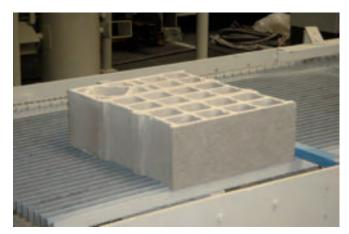
The highlight at this year's event was the Cutmaster presentation. A detailed report will follow in the next edition of CPI. The Cutmaster can make masonry blocks perfectly flat, so that they can be laid in a thin-bed adhesive without a mortar layer, making the construction more energy efficient.
