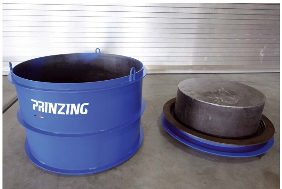
Fig. 2: The moulds are comprised of interior support core, steel pallet and mould jacket
