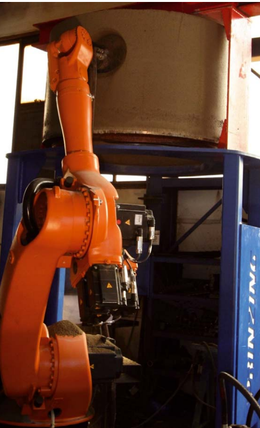
Fig. 5: Milling the connections on the milling centre
