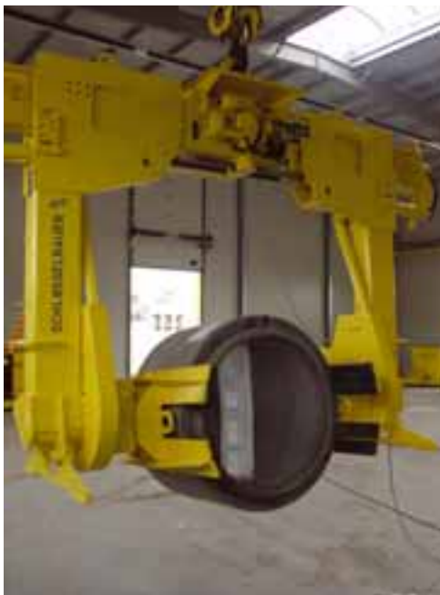
The Schlüsselbauer turning device turns cured manhole bases after removal of the moulds.
