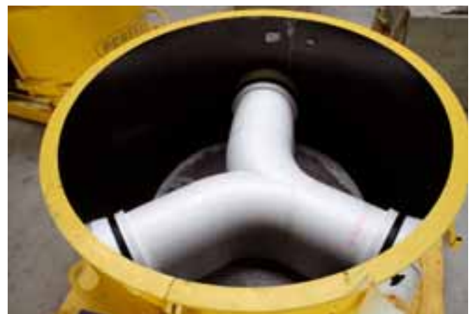
The prefabricated block-out element is mounted on top of the inner core and held in place by centring pieces, casting with usage of a central installed Putzmeister concrete pump.
