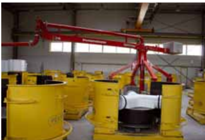
The prefabricated block-out element is mounted on top of the inner core and held in place by centring pieces, casting with usage of a central installed Putzmeister concrete pump.
