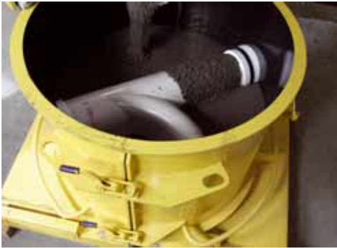
Manhole bases are manufactured using self compacting concrete, which is pumped into a mould by the Putzmeister pump.
