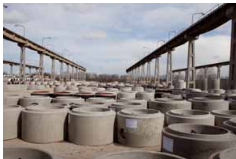
Manufacturing of monobases in one pour on the PERFECT system is the emphasis of Betonika plus s.r.o.
