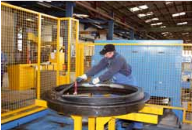
Installation of the gasket for products with an integrated seal
