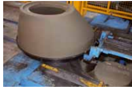
Production process: Pallets are fed, concrete poured into the mould and after the casting process the manhole riser is demoulded and pushed out of the production machine
