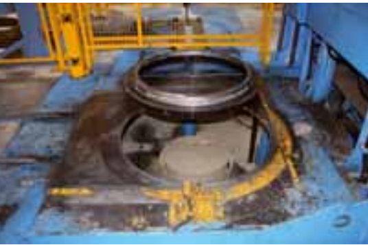
Production process: Pallets are fed, concrete poured into the mould and after the casting process the manhole riser is demoulded and pushed out of the production machine
