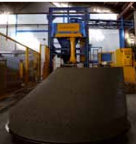
The green product in the "parking zone" prior to transport to the curing area
