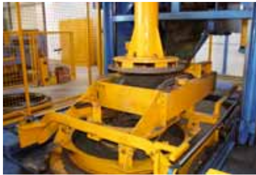
Production process: Pallets are fed, concrete poured into the mould and after the casting process the manhole riser is demoulded and pushed out of the production machine
