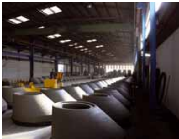
The green product in the "parking zone" prior to transport to the curing area
