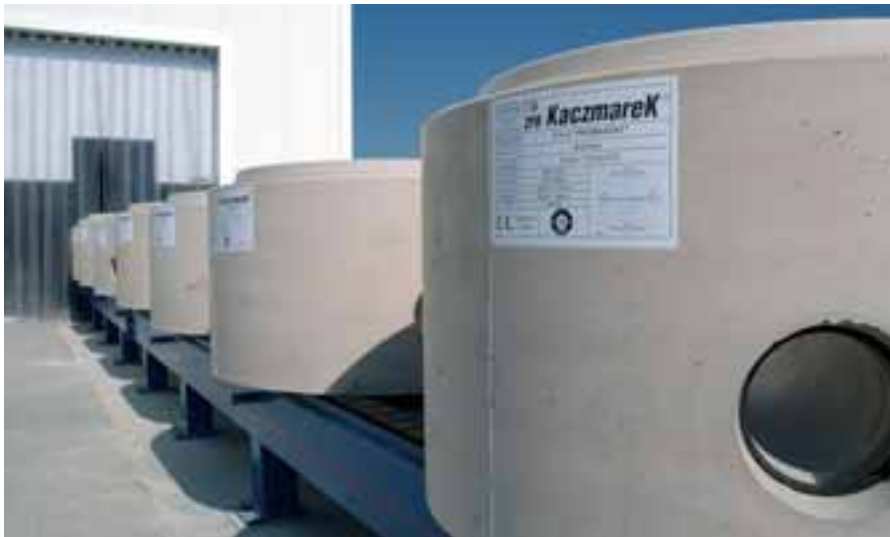
The labelling of each custom-made manhole base supports the whole logistic – also the installation on site.
