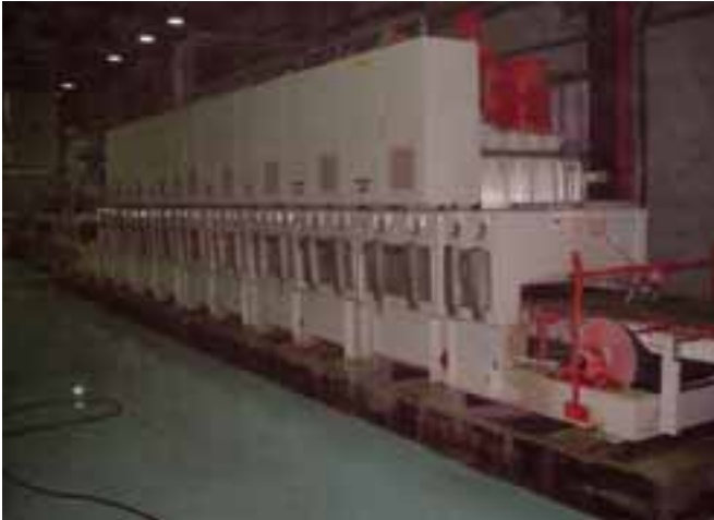
Star 8909 grinding machine for 2-rows of 40/40 cm slabs with drying section
