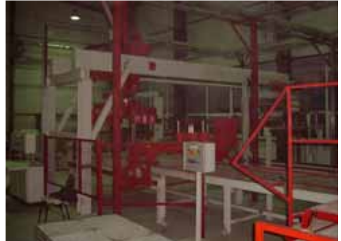
Transfer device for packing paving stone layers
