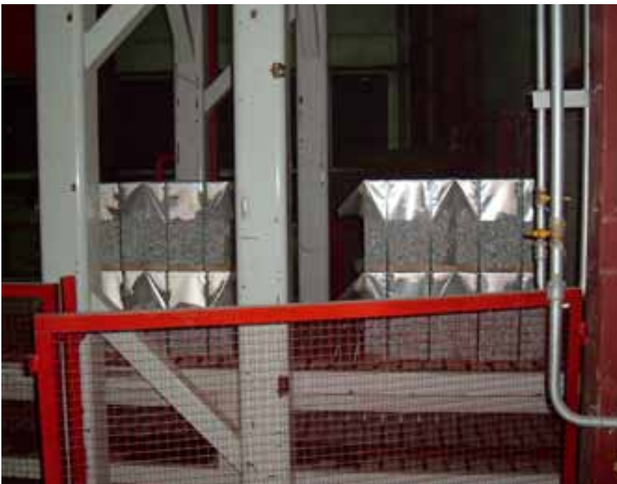
Double packages after passing through the cover sheet feeder and vertical strapping unit
