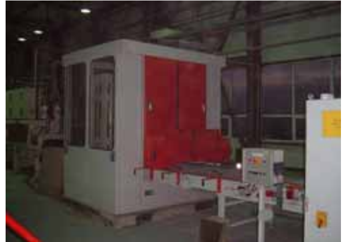
Bush hammering line with 6 rapid-change bars and a total of 87 bush hammers
