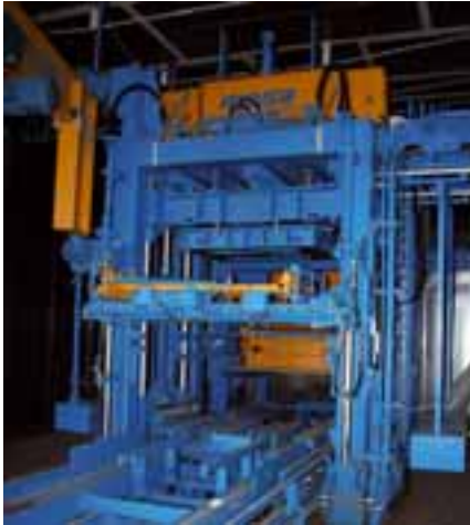
The concrete block machine Masa XL 9.1 is the heart of the plant
