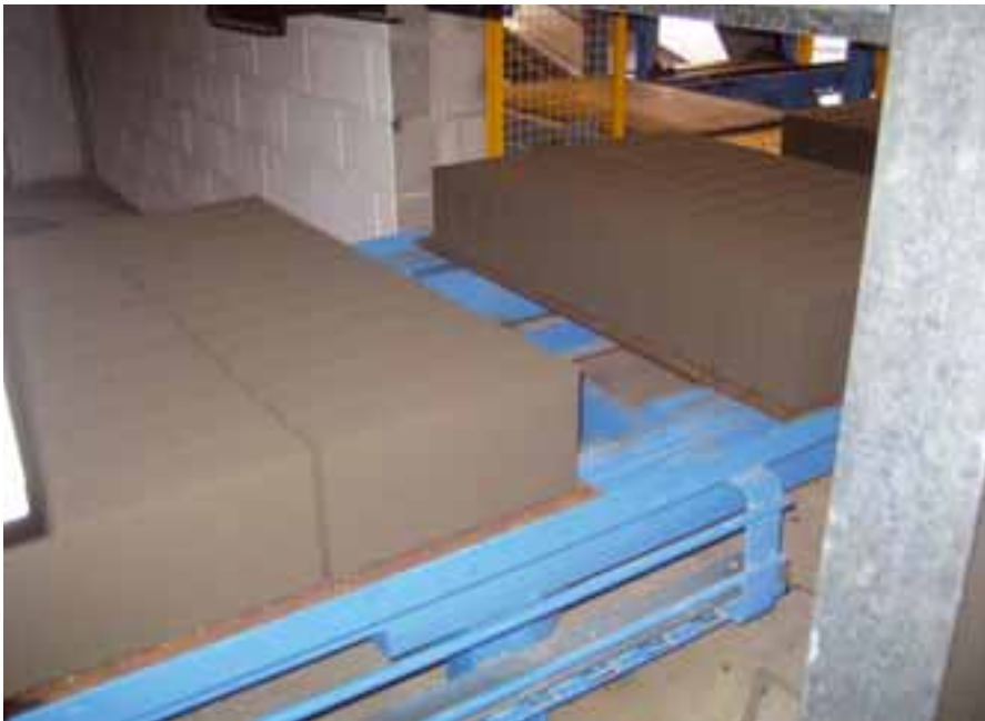
Production of 24 concrete blocks per cycle (440 x 215 x 100 mm)
