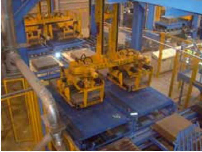
Depalletizing, remodelling and cubing
