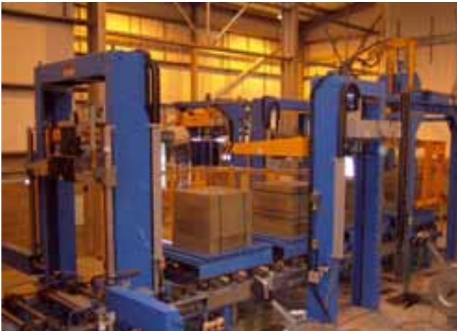
Strapping and handling of the cubes
