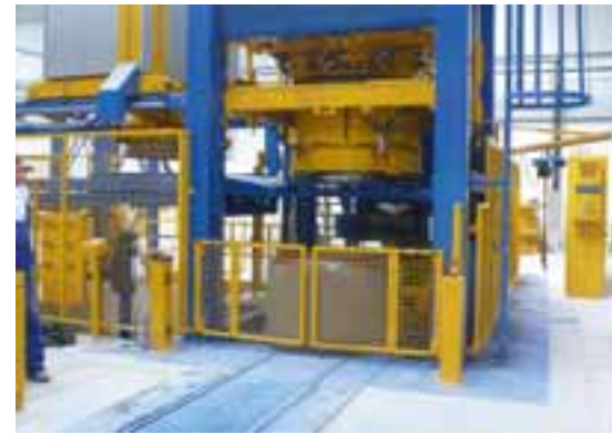
The Exact 1500 in operation – fully automatic production of manhole risers with top and bottom pallets
