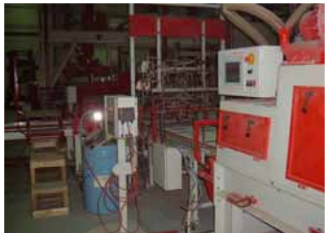
Impregnation with upstream curling machine
