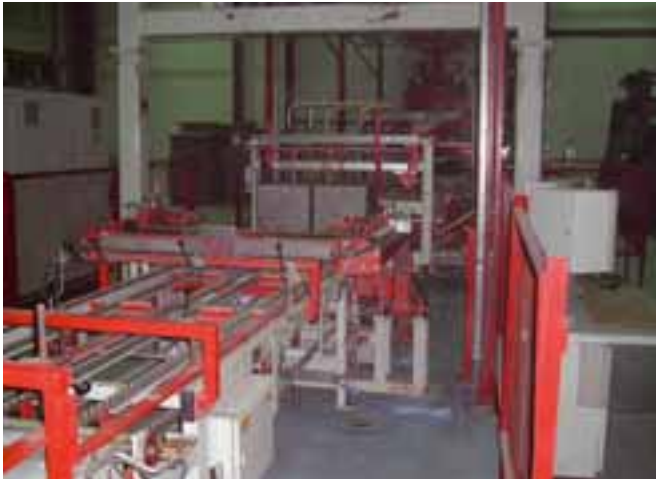
The 1st choice slabs are discharged after refinement via angled transfer units and belt conveyors to the vertical packing station.
