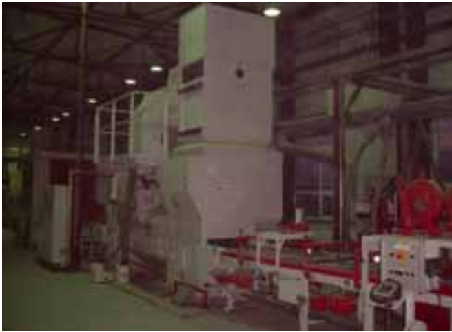
The shot blasting machine is equipped with 2 high-performance turbines, each rated at 15 KW.
