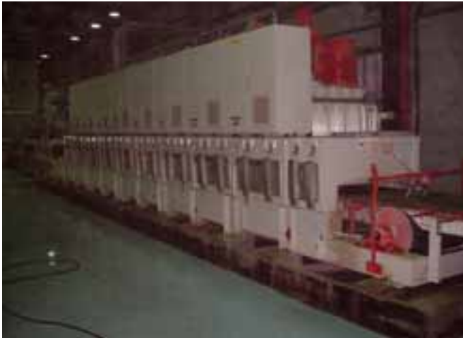
Star 8909 grinding machine for 2-rows of 40/40 cm slabs with dry-grinding section
