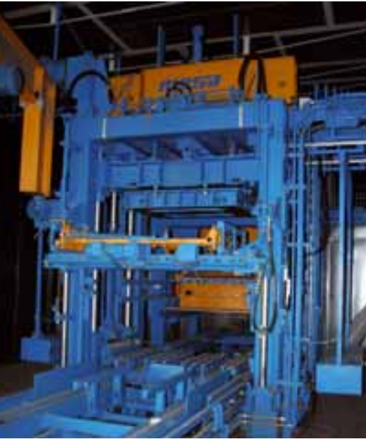
The concrete block machine Masa XL 9.1 is the heart of the plant
