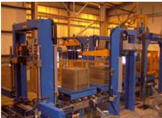
Strapping and handling of the cubes
