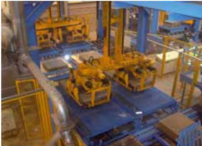
Depalletizing, remodelling and cubing
