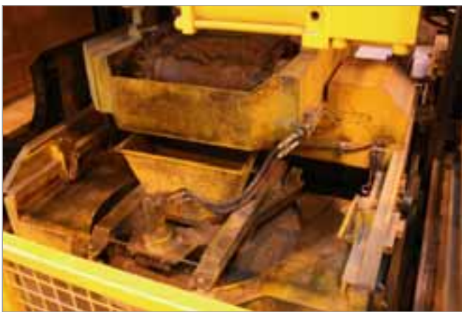
The concrete is transferred to the production plant via a conveyor.
