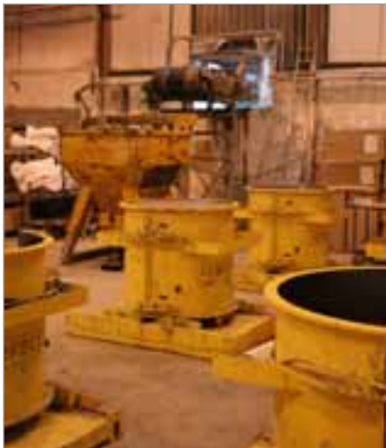
Via a conveyor the self-compacting concrete is transferred into the crane bucket which pours out the moulds.
