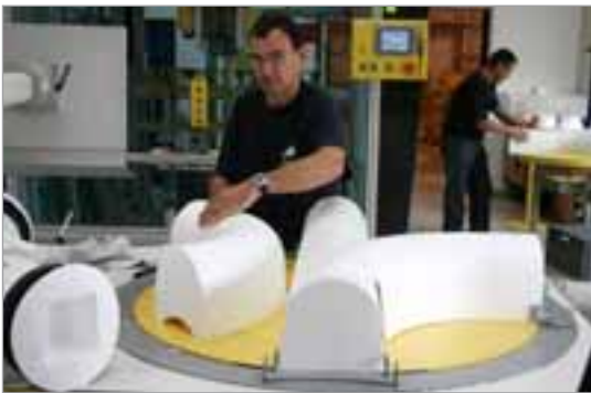
When preparing the production of the manhole bases, mould pieces are cut out of polystyrene by a hot wire so that all curves fit perfectly together when the individual parts are put together.
