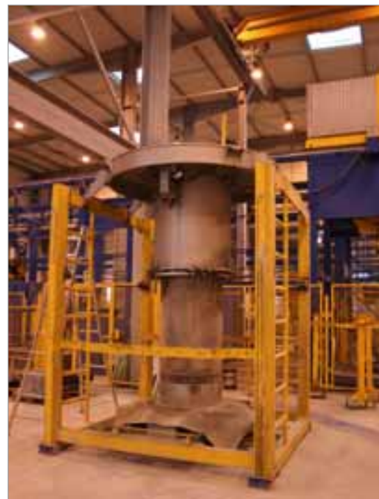
At a mould exchange the moulds are prepared in special boxes over-ground.
