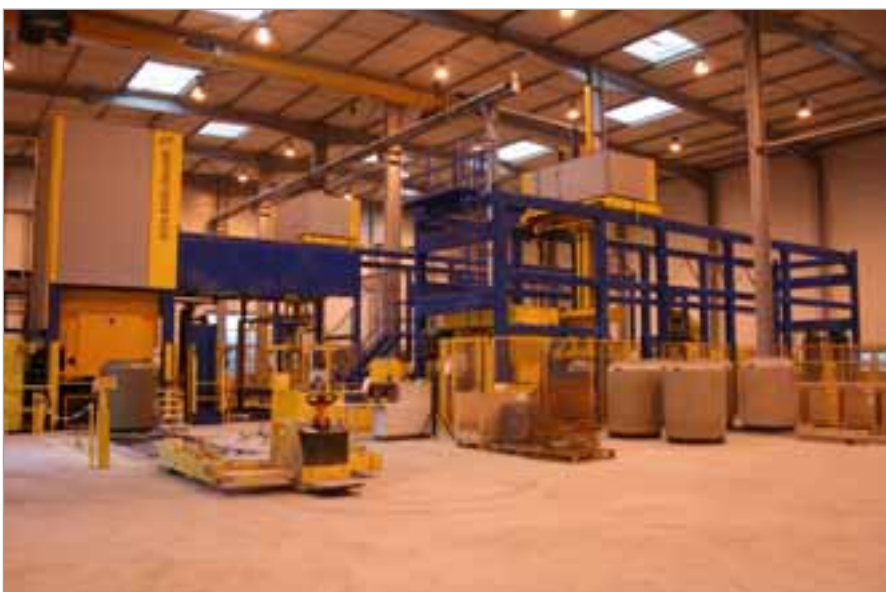
At Plattard in Villefranche, France, a brand-new Exact manhole production plant has been started up recently.
