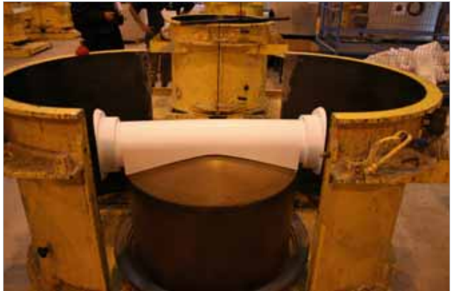
The finished mould parts are placed into the prepared moulds for the manhole bases.
