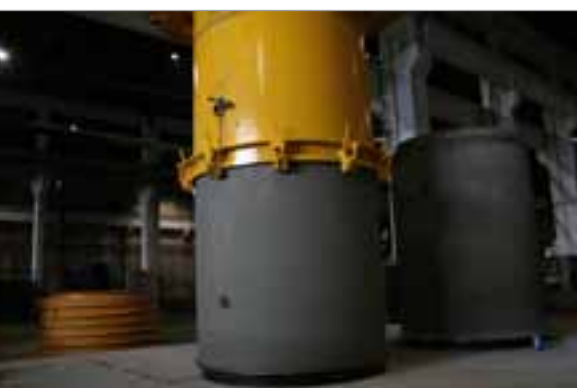
Outfeed of the filled mould out of the pipe station and its transfer to dismantling.
