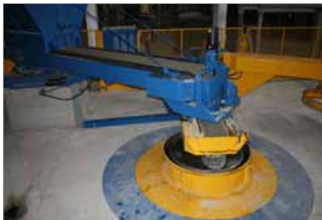
Two multi-movable feeding strips guarantee an exact insertion of concrete and adjustment to the product being manufactured – the duration of filling is optimized.
