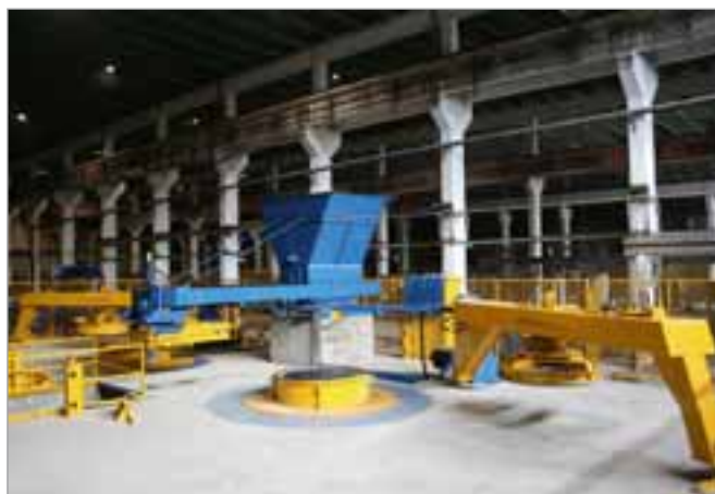
The production plant EXACT XL at a glance: In-between the two production stations for pipes and manholes the concrete box with its feeding strips and the operation panel are arranged.
