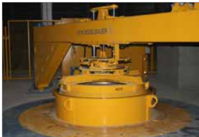
Each production station disposes of an independent pressing unit – here you can see it in use to finally shape a concrete pipe Ø 1600 mm.
