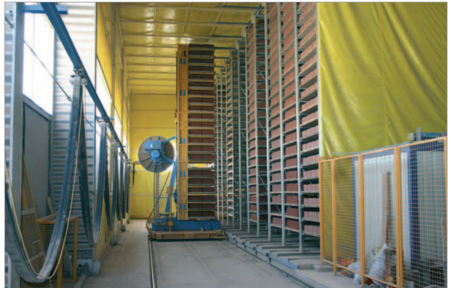
The fully automatic moving platform loads and unloads the shelving unit automatically
