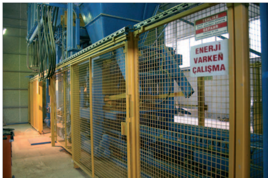
The block forming machine at Özkul is fenced off as required by safety regulations
