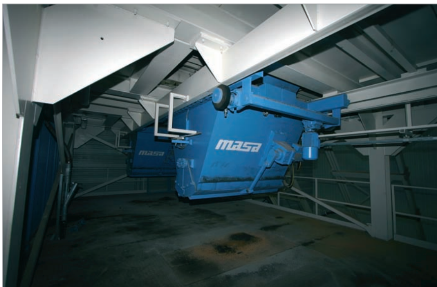
The twin bucket conveyor system has a total capacity of 6.400 l
