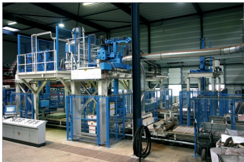
All movements are carried out with servo motors apart from the clamps
