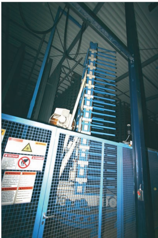
The products are brought to the dry side by means of a lifting frame, moving platform, drying shelf and lowering frame
