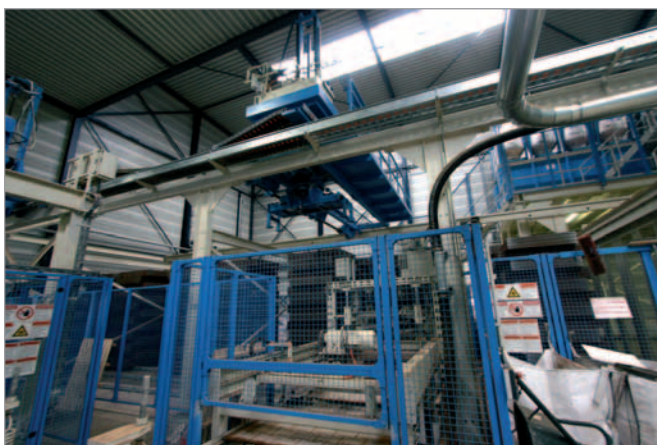
The pallet stacks are fed back to the block manufacturing plant using a sheet stacking crane
