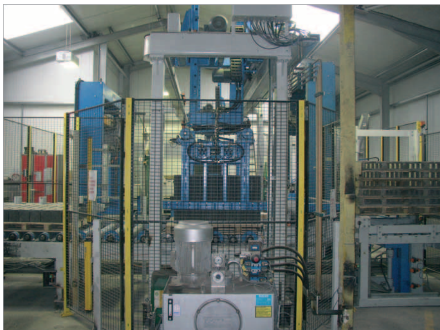
A four sided gripper takes the products from the pallet. The empty pallets (right in picture) are stacked for later use.
