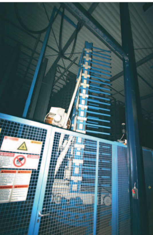
The products are brought to the dry side by means of a lifting frame, moving platform, drying shelf and lowering frame
