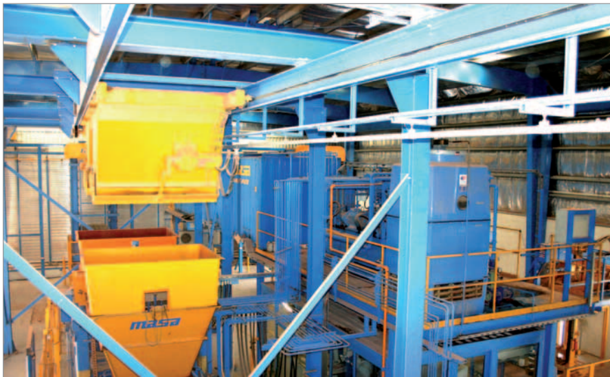
Block production machine and skip railway system at Bucomac – the cooling tower can be seen in the background on the hydraulic platform
