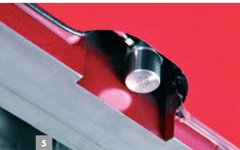
Kobra »Oscillate« – optional platform for carrying acceleration measurement sensors
