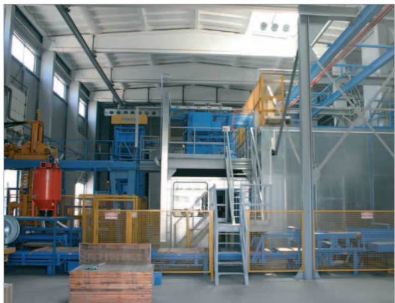
The Record 9001 VB block-making machine is completely insulated for reasons of noise protection.
