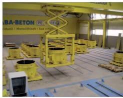
A view of the production of new "Perfect" manhole bases. Each manhole is manufactured with an individually formed channel using a special CNC controlled and contact-free hot wire cutting technology to precisely configure the required fittings. The precasting plant uses an automatic system for handling, crane transport and storage of the moulds for the manhole bases
