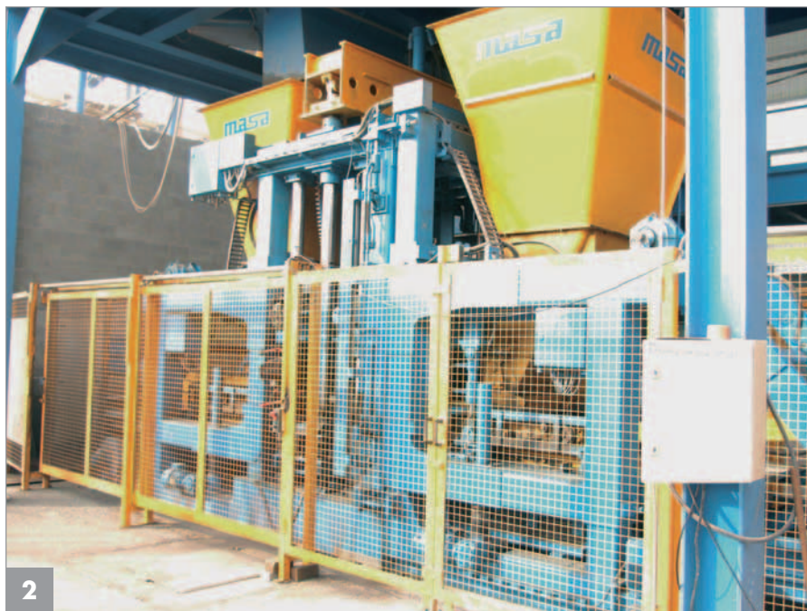
Stone manufacturing machine Record 9001 XL
