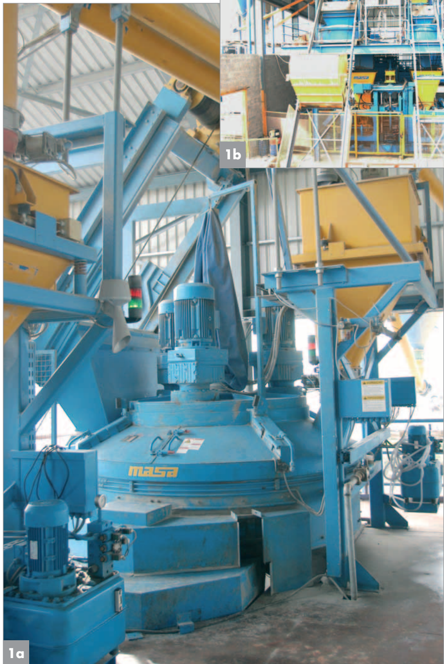
► The high power mixer HPM 2000/3000 in the plant at Ipsonas
