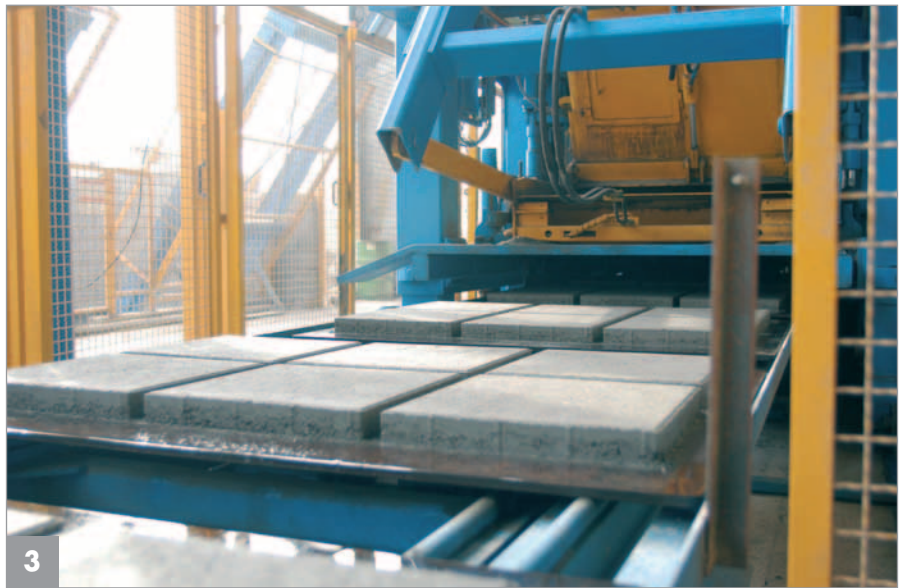
Production of concrete tiles on Masa 9001 XL
