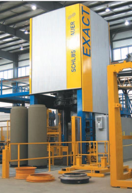
Twin production of the new 600 mm pipes
