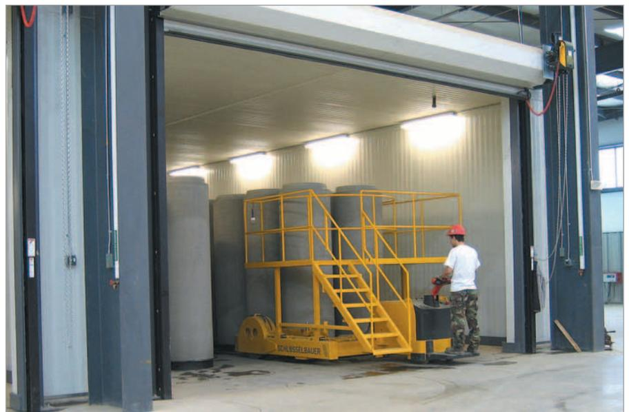
*Curing chambers for efficient curing of the pipes*
