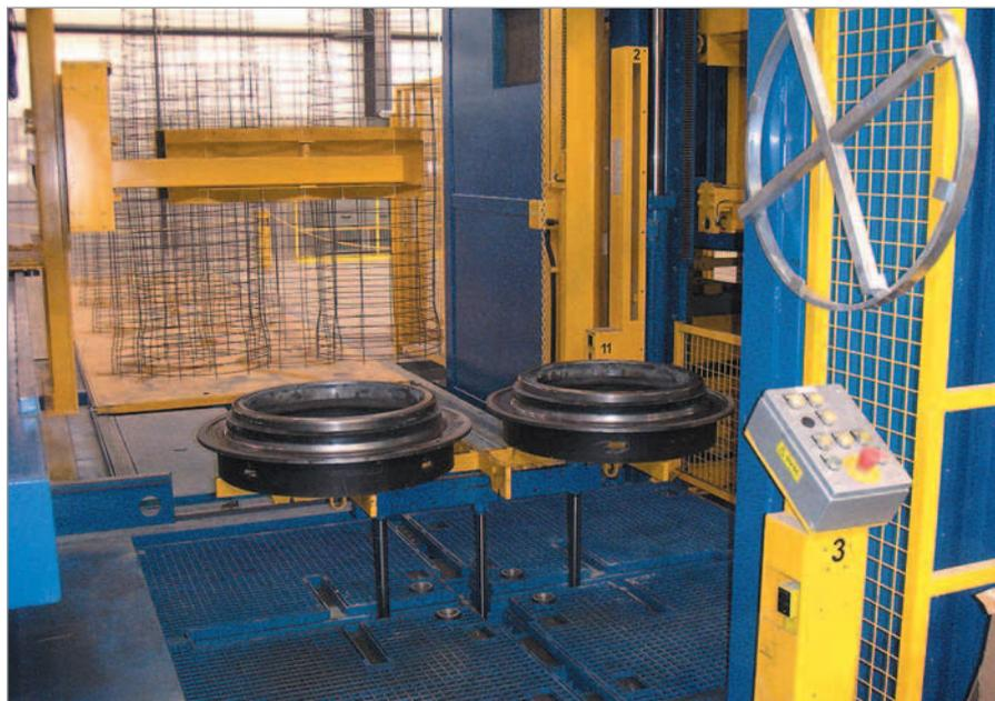
*Bottom pallets with the new integrated gasket*
