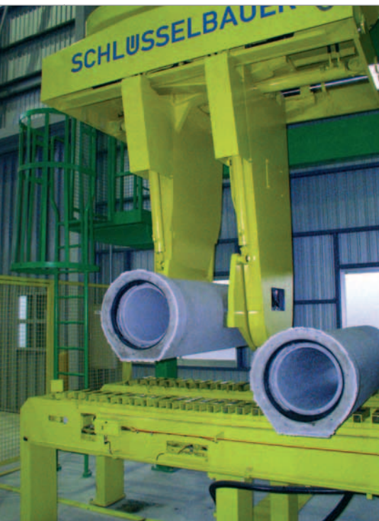
Automatic pipe manipulation
