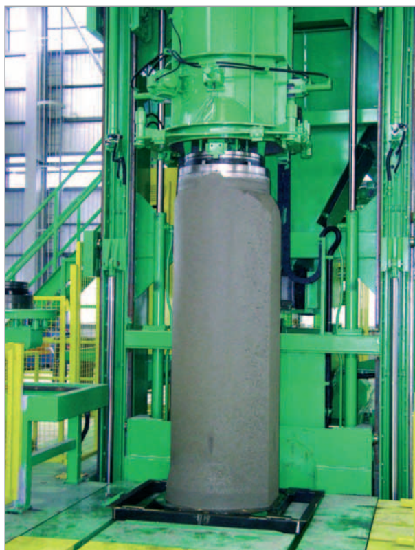
A freshly demoulded flat base pipe DN 600x2500mm
