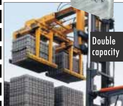
Forklift Attachment Double Grab with Telescopic Crane Boom DZ II
