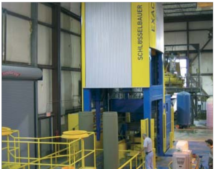
EXACT 2500 Pipe and Manhole production machine
